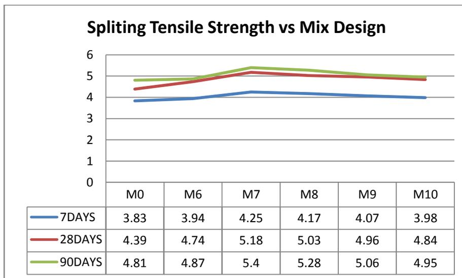
Fig.6 splitting tensile Strength vs. Mix Design of cement replaced by red mud for 7, 28 and 90 days
