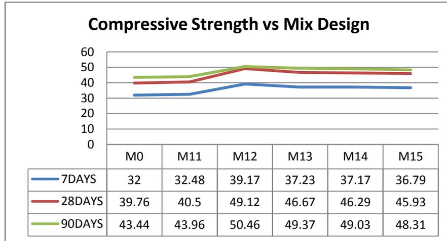
Fig.4 Compressive strength vs. Mix Design of replaced red mud and foundry sand for 7, 28 and 90 days
