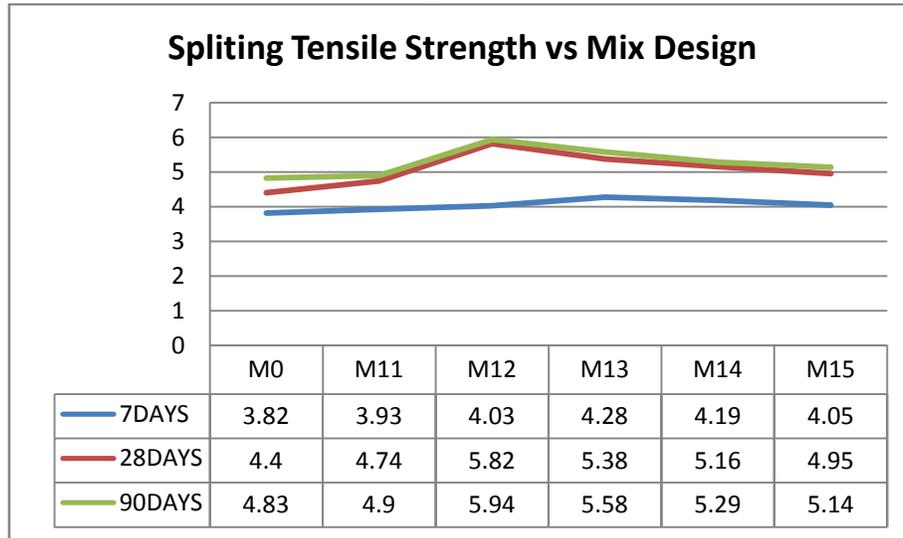
Splitting tensile Strength vs. Mix Design of replaced red mud and foundry sand for 7,28 and 90 days
