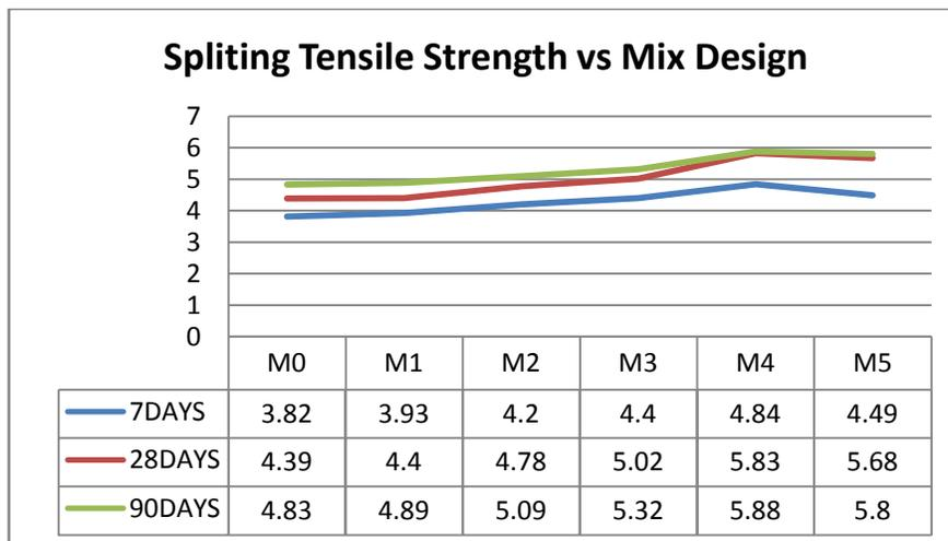
Fig.5 splitting tensile Strength vs. Mix Design of replaced foundry sand for 7, 28 and 90 days
