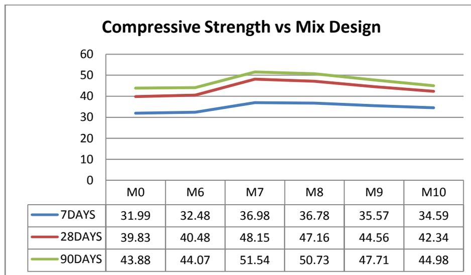
Fig.3 Compressive strength vs. Mix Design of replaced red mud for 7, 28 and 90 days W/C=0.48
