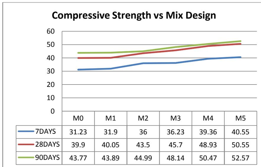
Fig. 2 Compressive strength vs. Mix Design of replaced foundry sand for 7, 28 and 90 days
