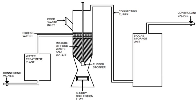
**Fig.2 Alternative design for biogas plant**
