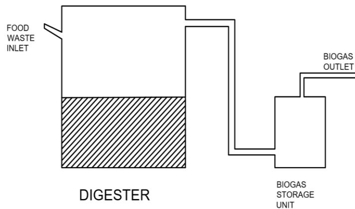
**Fig. 1: Conventional Biogas plant**
