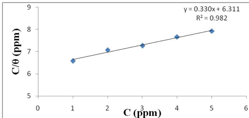
**Figure.4 – Langmuir adsorption isotherm plot for copper metal in 0.5 M HCl at 313 K in the presence of various concentration of *TerminaliaCatappa* leaf extract**
