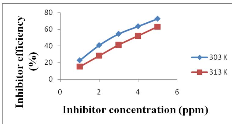
Figure.2 – Effect of concentration of *TerminaliaCatappa* leaf extract on inhibitor efficiency of copper metal in 0.1 M HCl at different temperature
