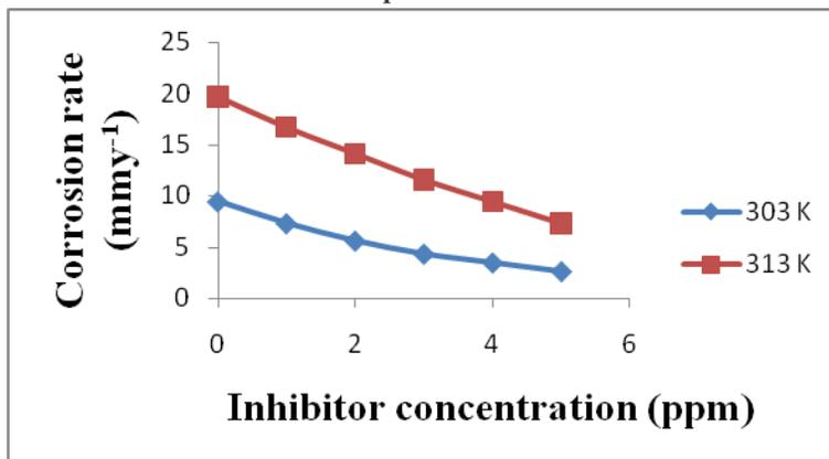
Figure.1 – Effect of concentration of *TerminaliaCatappa* leaf extract on corrosion rate of copper metal in 0.1 M HCl at different temperature
