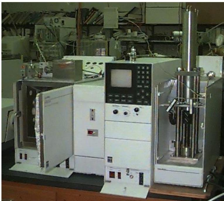
Figure 3: Supercritical Fluid Chromatography
