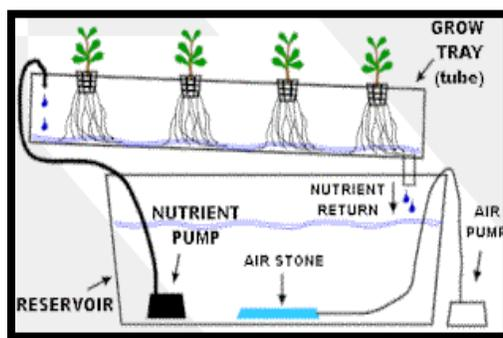
**Fig2.4.1. Nutrient Film Technique**
